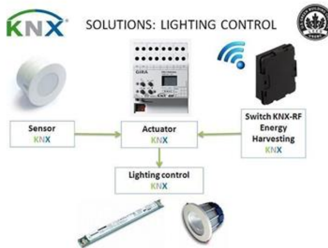
Figure 2.2: KNX Lighting System Component [6]
