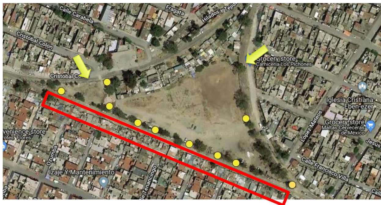
Figure 8: Yellow circles mark locations of solar street lights; Red box indicates community location; Arrows indicate access points to homes
